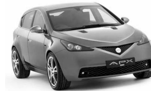
In addition to VVA, the APX also features a new 3 liter, super-charged V6 engine by Lotus Engineering. The power output is 300 bhp and the APX does 0-60 in 5 seconds. The engine is described as "production feasible" and also has normally aspirated and 2.2 liter displacement versions.
